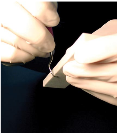
ROUNDING THE TOE STRAIGHT SICKLE
